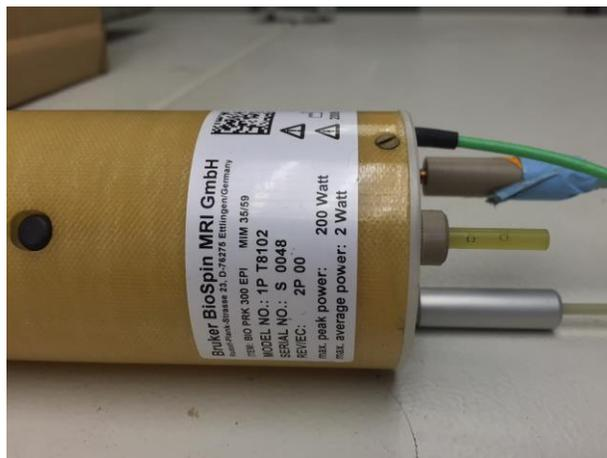
3)  $^1\text{H}$  72mm inner diameter, 112 mm outer diameter, 270 mm mechanical length, 110 mm symmetrical coil-center electrical length linear transceiver volume coil with active decoupling and 750W maximum transmit pulse of 5 ms.. Model T10720
