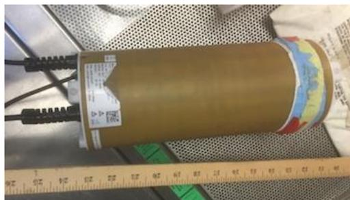
9)  $^1\text{H}$  105 mm x 60 mm x 25 mm receive-only mouse head coil array. Model T11765
