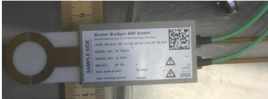
7)  $^1\text{H}/^{31}\text{P}$  Dual-tuned 300 MHz/121 MHz transceiver surface coil with 20 mm inner diameter. Model T6615
