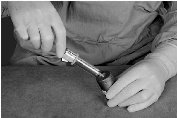
Fig. E.3. Positions of hands used for dispensing radiopharmaceutical with the vial tipped at 45° over a bench and withdrawing liquid using a longer syringe needle (Martin and Whitby, 2005) (with permission from Lippincott Williams and Wilkins).
